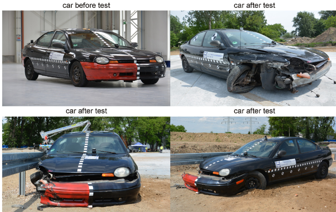
Fig. 11 – Photos of Dodge Neon car used in TB32/CBC test.
