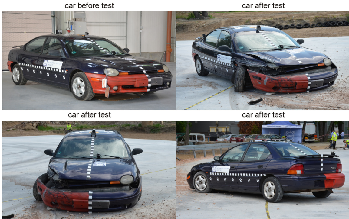
Fig. 7 – Photos of Dodge Neon car used in TB32/CB test.
